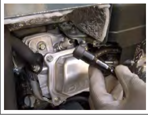
11.5.2-11 Spark plug check - Step 1.
