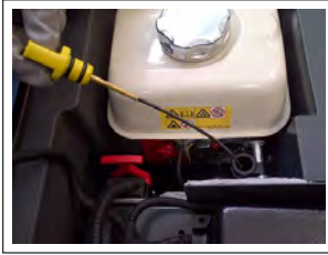
11.5.2-2 Oil Level check - Step 2.
