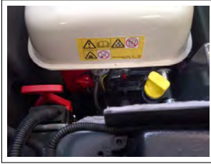
11.5.2-1 Oil Level check - Step 1.
