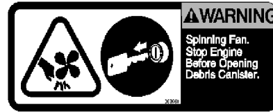
MOVING FAN HAZARD LABEL- Located On The Debris Canister.
