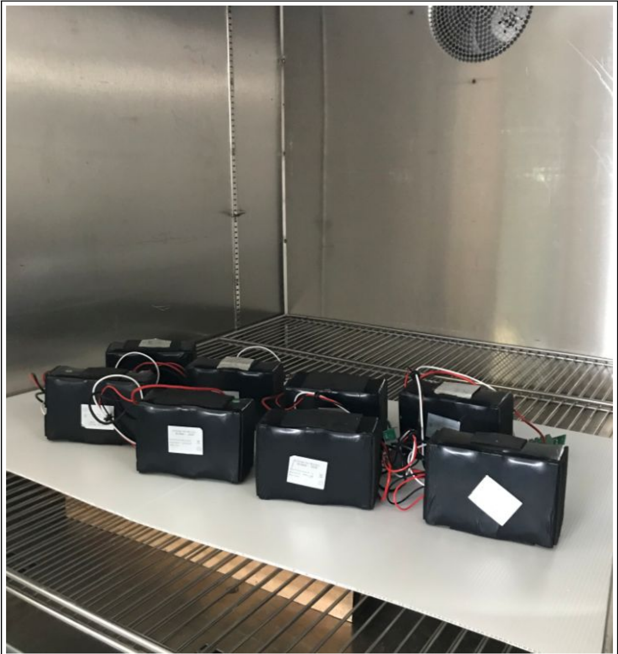
Fig. 2.2 Batteries in T.2 Ref.1 and Ref.2b, §7.2.2 Ref. 2a Test setup (Thermal test, case stress)
