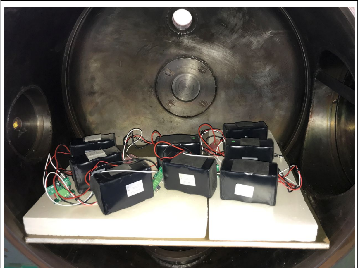
Fig. 2.1 Batteries in T.1 Ref.1 and Ref.2b Test setup (Altitude Simulation test)
