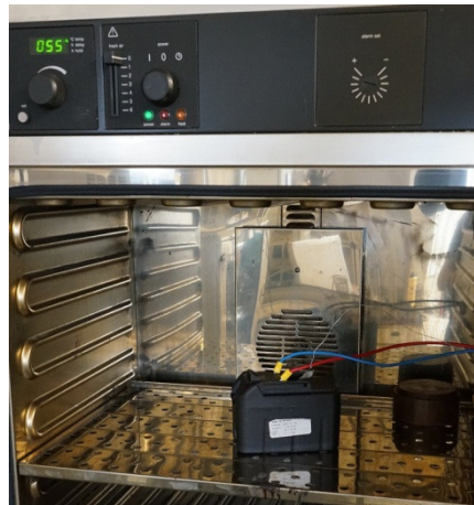
Figure 9: Short-circuit test in heat cabinet at 55 °C with the batteries
