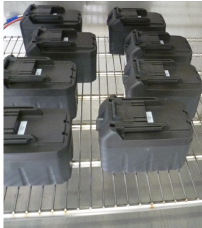
Figure 3: Thermal test in climate cabinet with the batteries inside
