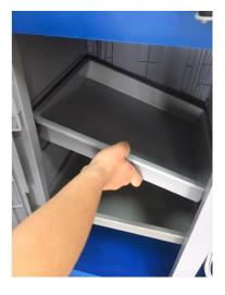
8 -Fixing top shelf and garbage cover on the column with scew by using scew driver.
