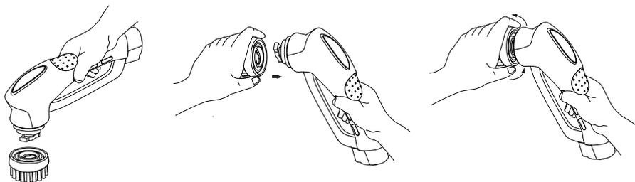
2. Open the battery cap on the bottom of the handle, put in the battery and then put back the cap.
