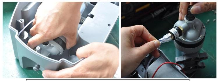
To take out the pump from the housing, disconnect the wire from pressure switch
