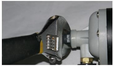
4). Screw the male connector to the female connector on the motor base. If it is not firmly, use a spanner.
