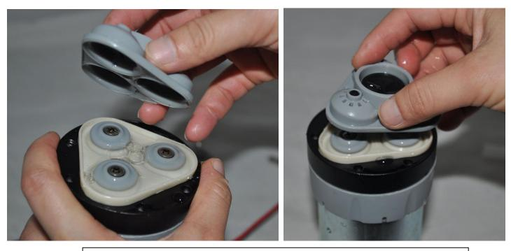
Replace the diaphragm seal and then assemble the pump cap back to the pump.
