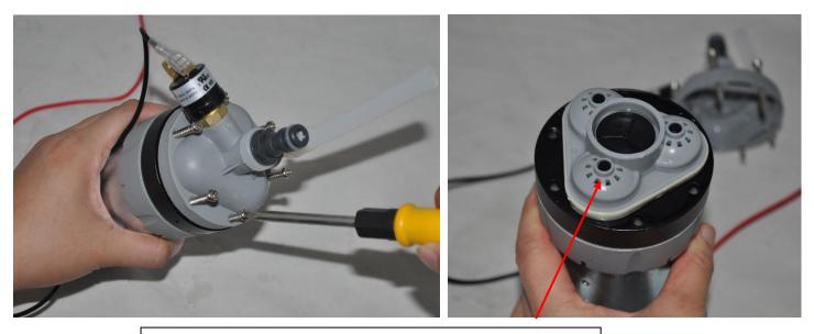
Unscrew the pump cap, see the diaphragm seal in the middle
