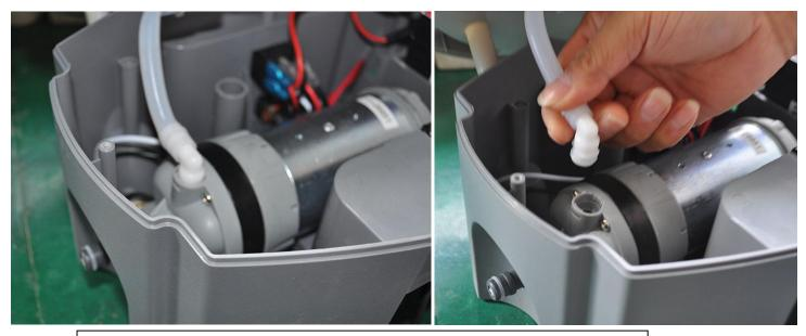
After open the upper cover, twist off the hose which is connected the pump
