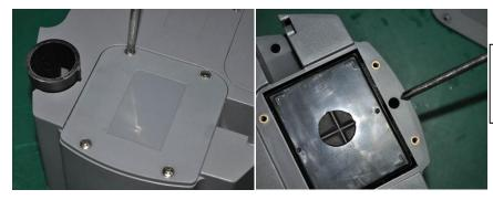
1pc inside the battery housing under the battery cover
