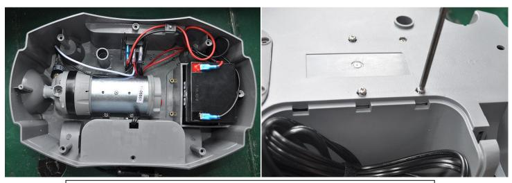
Unscrew the four screws on the bottom to release the pump from the housing
