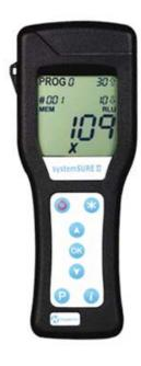
Clearing performance can be quickly assessed with the Bioluminometer.
