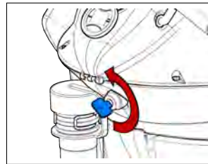
10.2.3-1 Machine switching off
