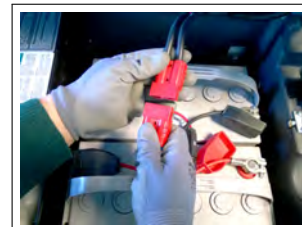
10.2.3-3 Unplug of battery connector
