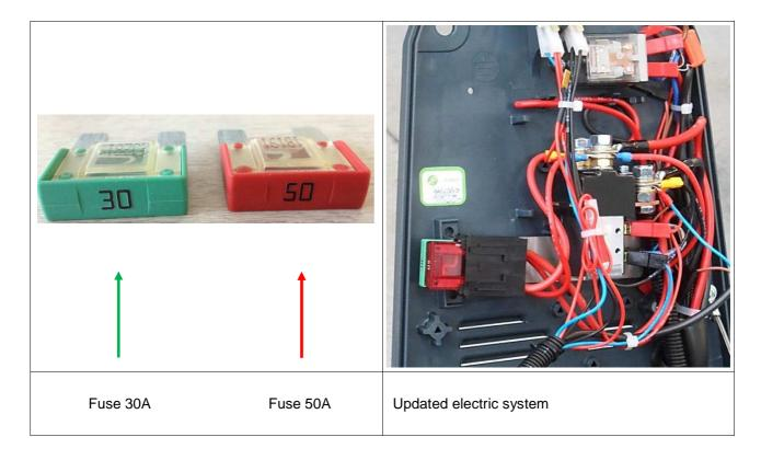
Note: The new fuse can be installed on previous models as well
