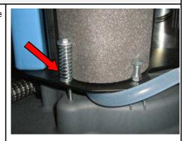
2. Tighten the **screw of the traction spring** so that it gets out to maximum of 0.5 mm from the **locking nut**.
