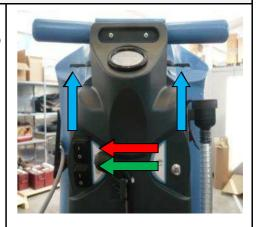
2. Check the battery contacts and the cable connection with the faston in the contactor mounted inside the machine handle.
