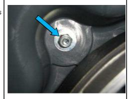
3. Tighten the **direction screw** so that it touches the plaque of the brush base. Unscrew it until there is a maximum gap of 1 mm between the bottom of the screw and the plaque of the brush base.
