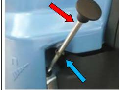
2. In the case of poor water flow, check the cleanliness of the cap.
