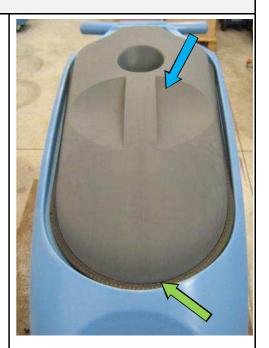
Check the cleaning and functionality of the filter with ball
