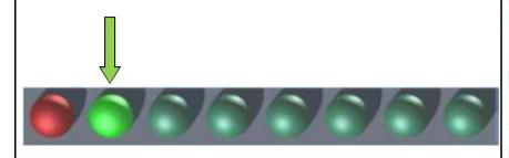
Make sure that with gel batteries the rotating microswitch is set to **position 4**, in this case the fourth LED will light.
