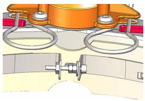
Picture 13: Front blade fixation
