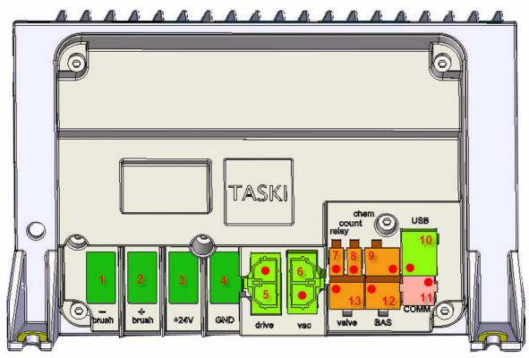
Picture 7: Power electronics connector
