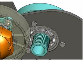
Picture 41: Intermediate pulley
