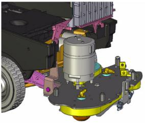
Picture 31: Brush drive replacing
