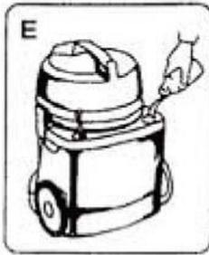
**E- Spray Extraction Liquid Tank Connection Hose** - Push the plug connector on the connection hose in to the corresponding aperture in the hood as far as it will go. Take care to ensure that the hose is not kinked and that the end of the hose with the strainer is positioned at the bottom of the tank. Spray extraction liquid. Remove the screw plug from the tank and pour in the mixture of water and concentrated cleaning agent with the aid of the funnel. The capacity of the tank is 4.5 liters.
