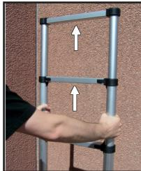
Please note that, while extending the telescopic ladder beginning with the top rung, the ladder is not locked and retracts if not all rungs are extended.
