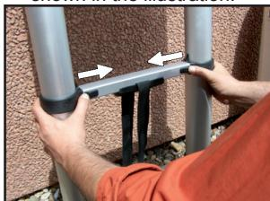
Start retracting the telescopic ladder at the highest rung you can reach, if the telescopic ladder was extended to its full length.
