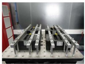
Set-up with batteries on slip plate (top view)
