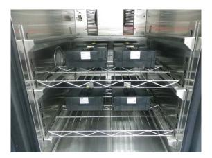
Batteries inside temperature chamber
