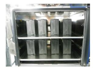
Batteries inside altitude chamber
