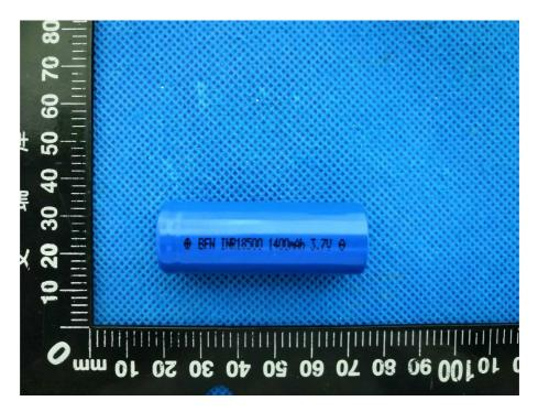
Figure 9 Front view of cell (18500 1400mAh)
