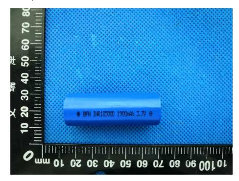
Figure 15 Front view of cell (18500 1900mAh)
